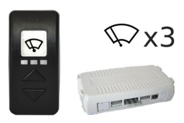
Control system for three wipers suited for high power motors. This system consists of the control switch and a relay box. It replaces up to three standard switches and it's suited for high power motors provided with parking switch. It works either with single speed motor and with double speed motor. Three buttons in the switch allow to manage all the functions needed for windscreen cleaning: ON/OFF, timing and washing program.
