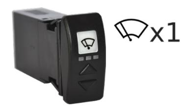
Control system for one wiper suited for low power motor. It's an all in one system, it doesn't need additional relay boxes, that makes it easy to mount (no screws are needed). It replaces up to two standard switches and it's suited for low power motors provided with parking switch. It works both with single speed and double speed motors. Three buttons in the switch allow to manage all the functions needed for windscreen cleaning: ON/OFF, timing and washing program.
