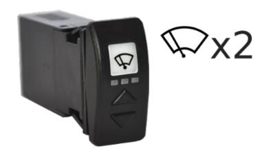
Control system for two wipers suited for low power motors. It's an all in one system, it doesn't need additional relay boxes, that makes it easy to mount (no screws are needed). It replaces up to three standard switches and it's suited for low power motors provided with parking switch. It works both with single speed and double speed motors. Three buttons in the switch allow to manage all the functions needed for windscreen cleaning: ON/OFF, timing
